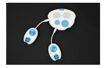
[Figure Caption:] This photo shows the Code Jumper Hub with a Play pod connected to Port 1 and another Play pod connected to Port 2.
